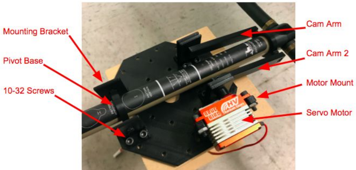
Figure 1: Final Assembly of Antenna Gimbal
